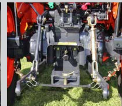
A rear lift capacity of 1131 kg. Standard with 2 sets of rear hydraulic remotes.
