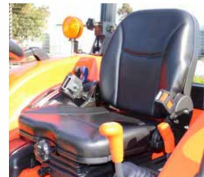
Adjustable mechanical suspension seat making operation more comfortable.
