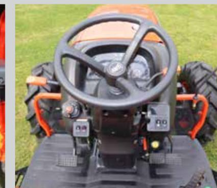
A flat operator station, with a tilt steering column and ergonomically placed controls.
