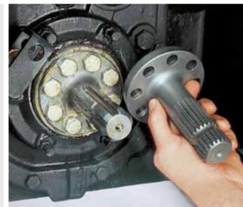
Fast replacement: The screw-connection PTO stub.
