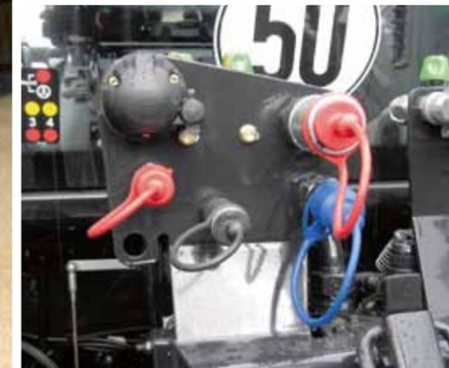
To order the Agrotor M can be fitted with Power-Beyond connectors for the direct connection of third-party devices.
