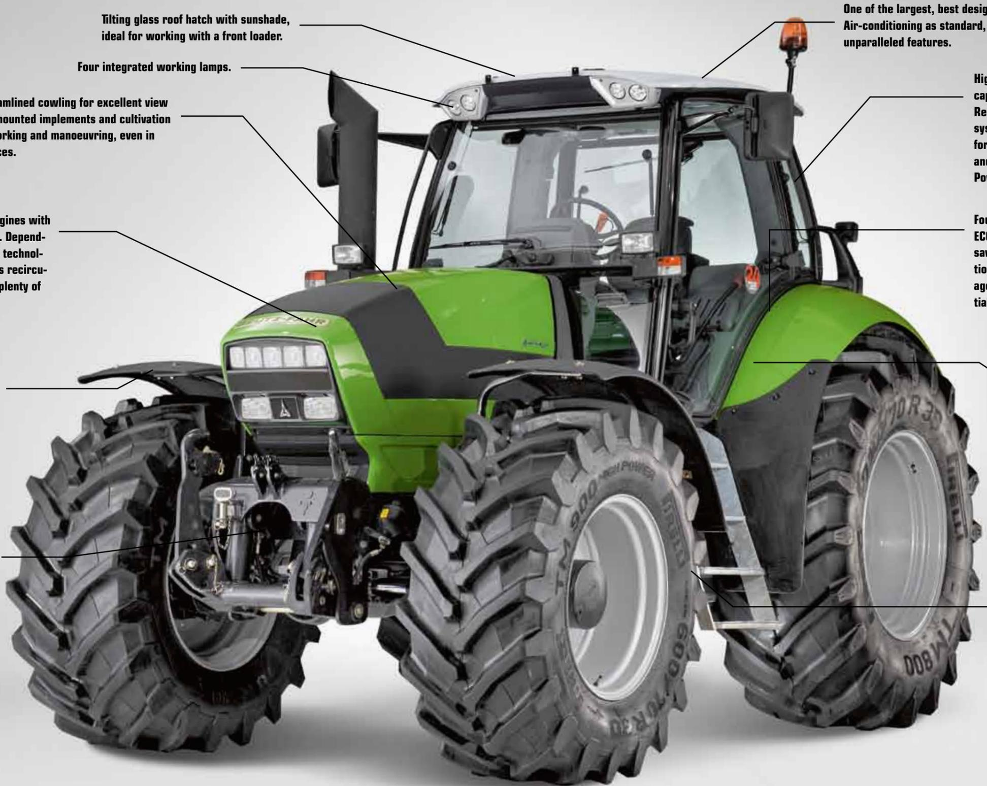
Tilting glass roof hatch with sunshade, ideal for working with a front loader.
