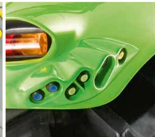
The rear controls on the ProfiLine versions can include controls for an additional remote valve to order.
