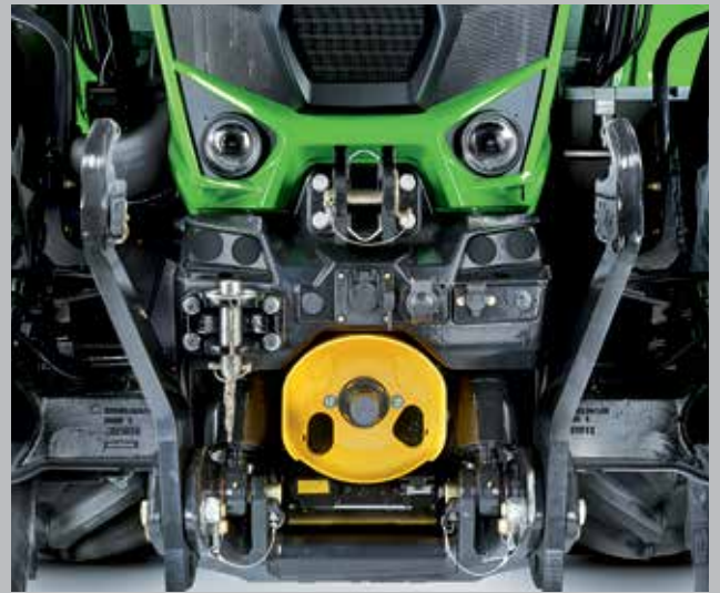
New front lift position control (TTV models) with maximum lifting power of 5,480 kg.
