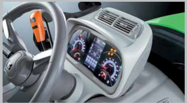
State-of-the-art dashboard cluster with new InfoCentre Pro : 5" high-res LCD colour display for customisable top information concept.
