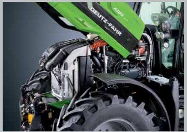
Highly efficient and compact cooling system with intercooler, engine, transmission, fuel cooler, and air conditioning condenser.
