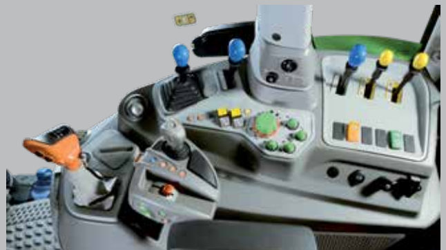
Ergonomic right hand control panel for Powershift version.
