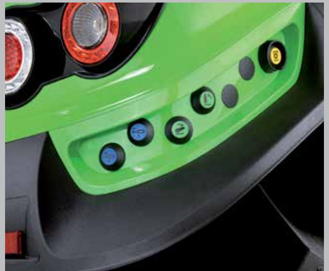
External hydraulic, rear power lift and PTO shaft can be easily controlled from each side.
