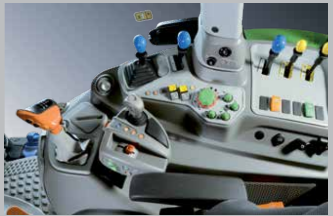
Powershift transmission: efficient all-round transmission with manual gear changing.
