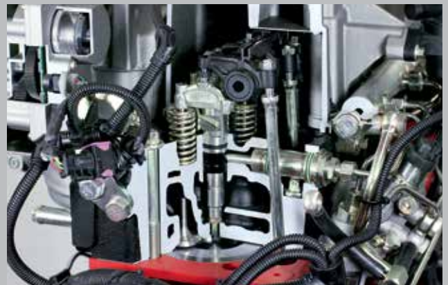
DCR technology. 1,600 bar injection pressure ensures maximum engine efficiency.
