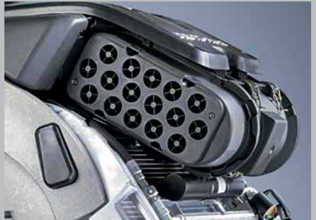
Precleaning system of the air intake filter: spiral cyclone tubes and an aspirator hose removes 95% of the dust before entering the primary filter.
