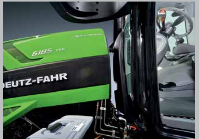
The cab and engine bonnet are separated from each other to significantly reduce noise and vibrations and thereby ensure maximum comfort.
